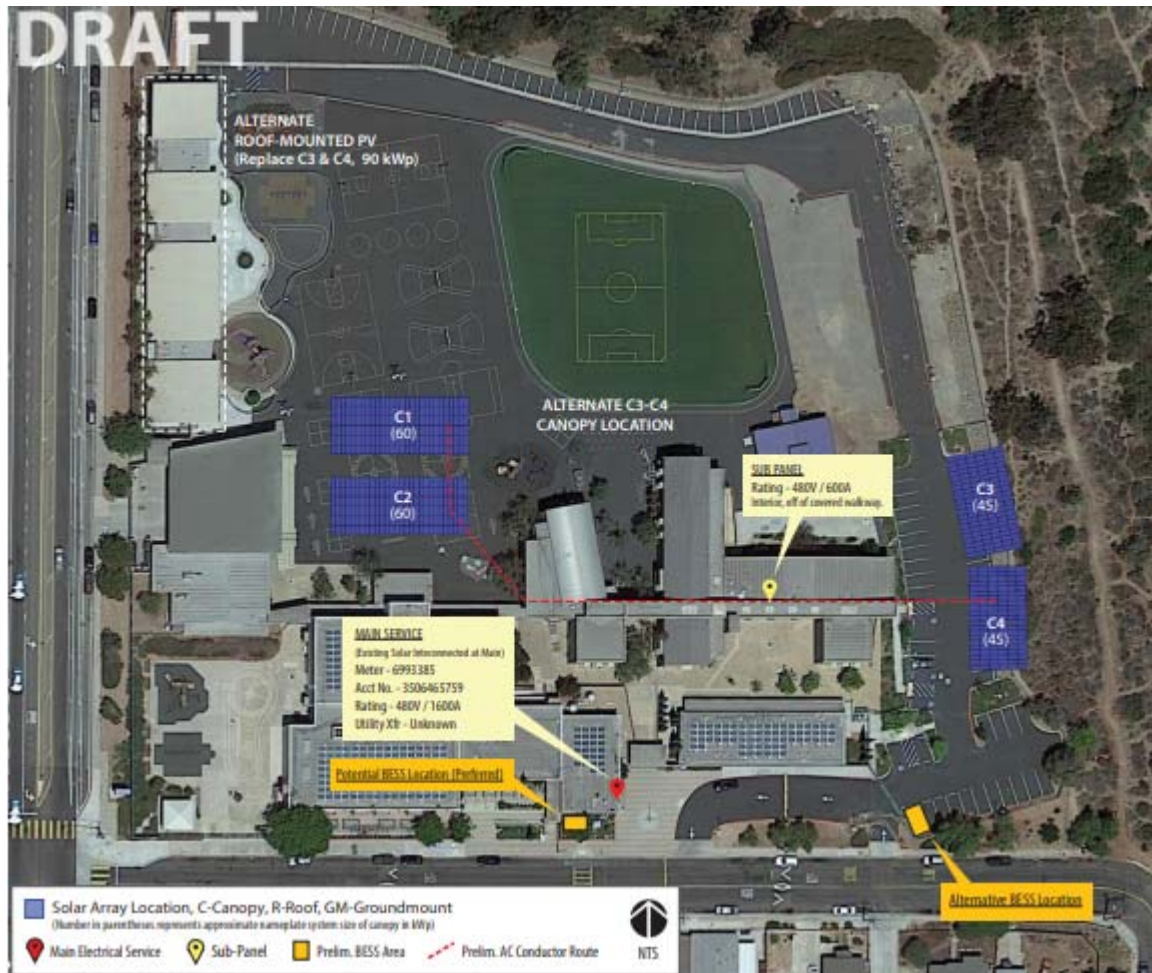
Proposed solar array placement
