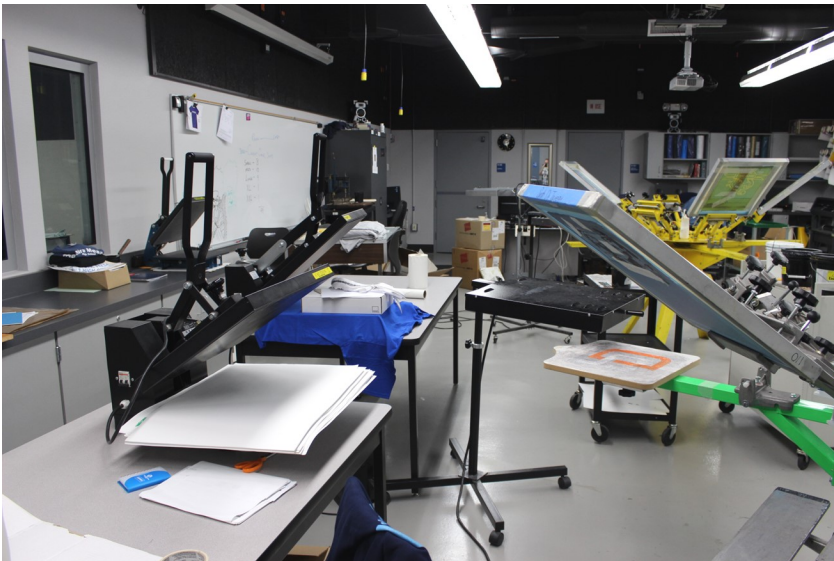
Heat press transfer machine station
